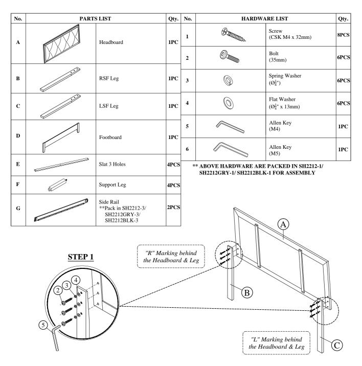
DO NOT TIGHTEN BOLTS UNTIL COMPLETELY ASSEMBLED.
