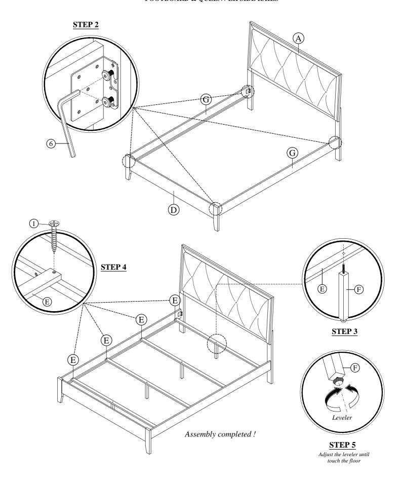
DO NOT TIGHTEN BOLTS UNTIL COMPLETELY ASSEMBLED.
